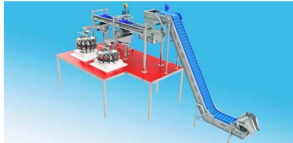
The production line, which will support Nutradia's drive to produce healthier, non-fried snacks, includes Fabcon's modular horizontal motion and vibratory conveyors that can be extended to support further packaging stations at the central Belgium factory.
